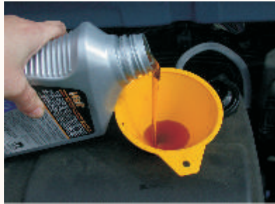
Fig: Fill up oil with funnel
