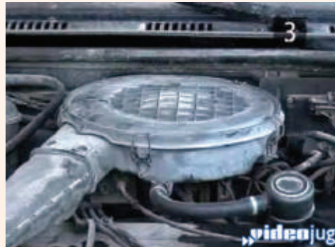
Fig : Cleaning of air filter housing
