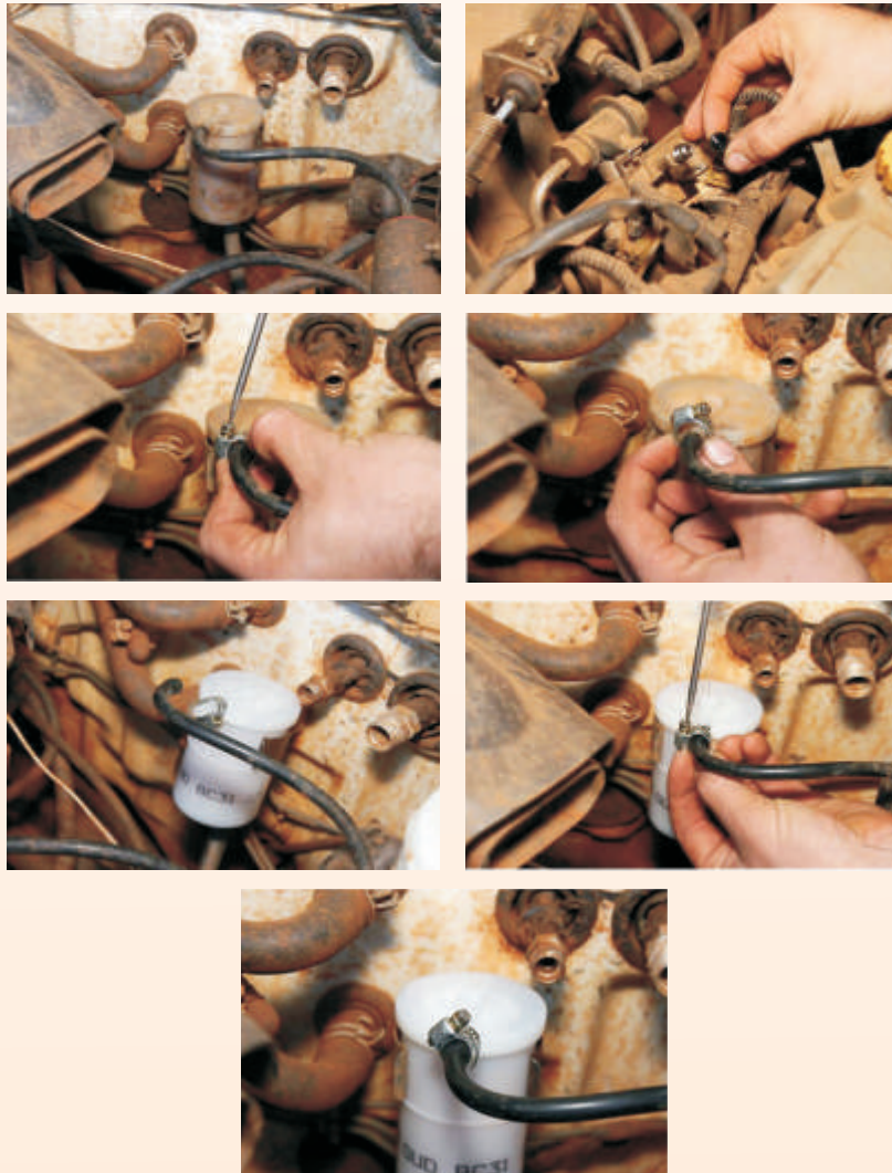
Fig: Photographs of Replacing Fuel Filter
